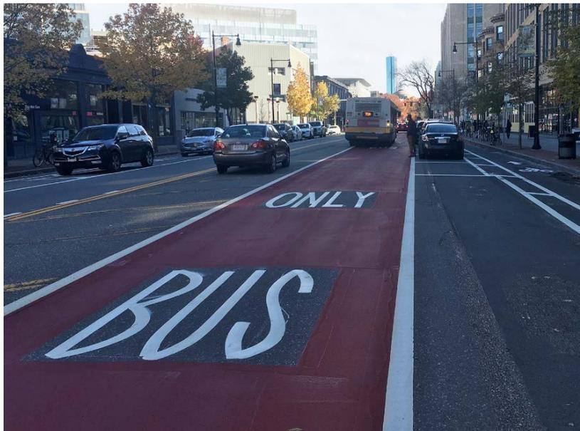
Figure 2 – Red pavement markings on Mass Ave in Central Square, Cambridge
