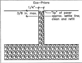
\*Note: Both maintenance types will be most effective when the joint aggregate material is filled to the "lip" of the paver. If the joint material has settled more than the joint width, plus 1/8 inch below the paver lip, the maintenance equipment is significantly less effective and potentially more expensive.
