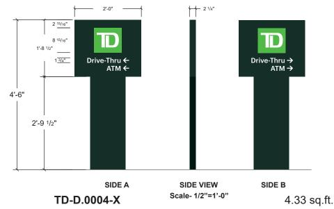
Non-illuminated painted directional sign with film decorated sign face. Aluminum tube frame and aluminum sheet construction. Sign to be painted to match: PMS 5535 #MP62874V1.0 (Satin Finish). Sign face first surface film 3M 5000 Scotchlite Reflective White Vinyl and 3M IJ680-10 Scotchlite Reflective Film (InkJet Digital) to match Matthews Pantone 361 with 3M MCS approved inkjet inks.
