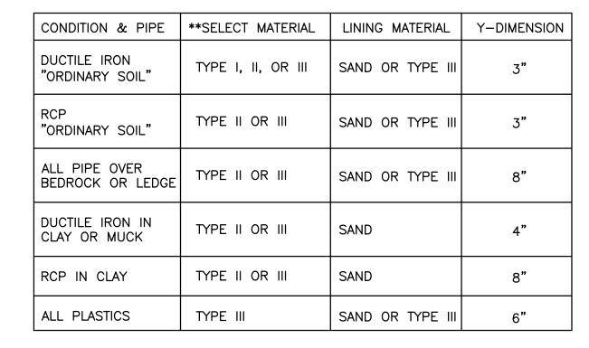
\* SUITABLE MATERIAL SHALL CONTAIN NO STONE GREATER THAN 4" IN DIAMETER, NO FROZEN LUMPS, AND ONLY MINOR AMOUNTS OF CLAY OR ORGANIC MATERIAL. ALL MATERIAL TO BE PLACED IN MAX 12" LIFTS AND COMPACTED BEFORE PLACING NEXT LIFT.
