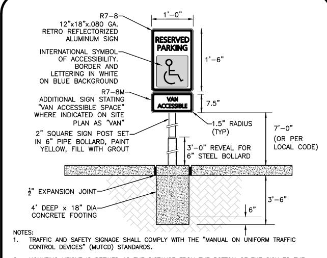
2. MOUNTING HEIGHT IS DEFINED AS THE DISTANCE FROM THE BOTTOM OF THE SIGN TO THE NEAR EDGE OF THE PAVEMENT. 3. PROVIDE ONE (1) SIGN PER ACCESSIBLE SPACE. SEE SITE PLAN FOR EXACT LOCATION.
