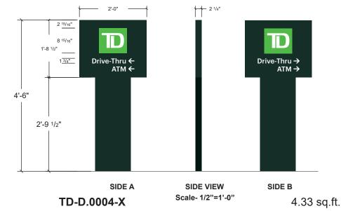
Non-illuminated painted directional sign with film decorated sign face. Aluminum tube frame and aluminum sheet construction. Sign to be painted to match: PMS 5535 #MP62874V1.0 (Satin Finish). Sign face first surface film 3M 5000 Scotchlite Reflective White Vinyl and 3M IJ680-10 Scotchlite Reflective Film (InkJet Digital) to match Matthews Pantone 361 with 3M MCS approved inkjet inks.
