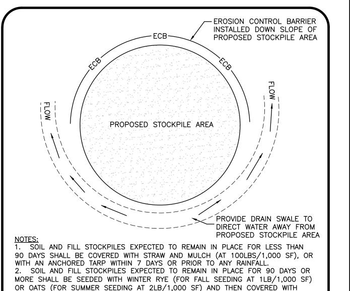
PRIOR TO ANY RAINFALL. STOCKPILE PROTECTION DETAIL NOT TO SCALE
