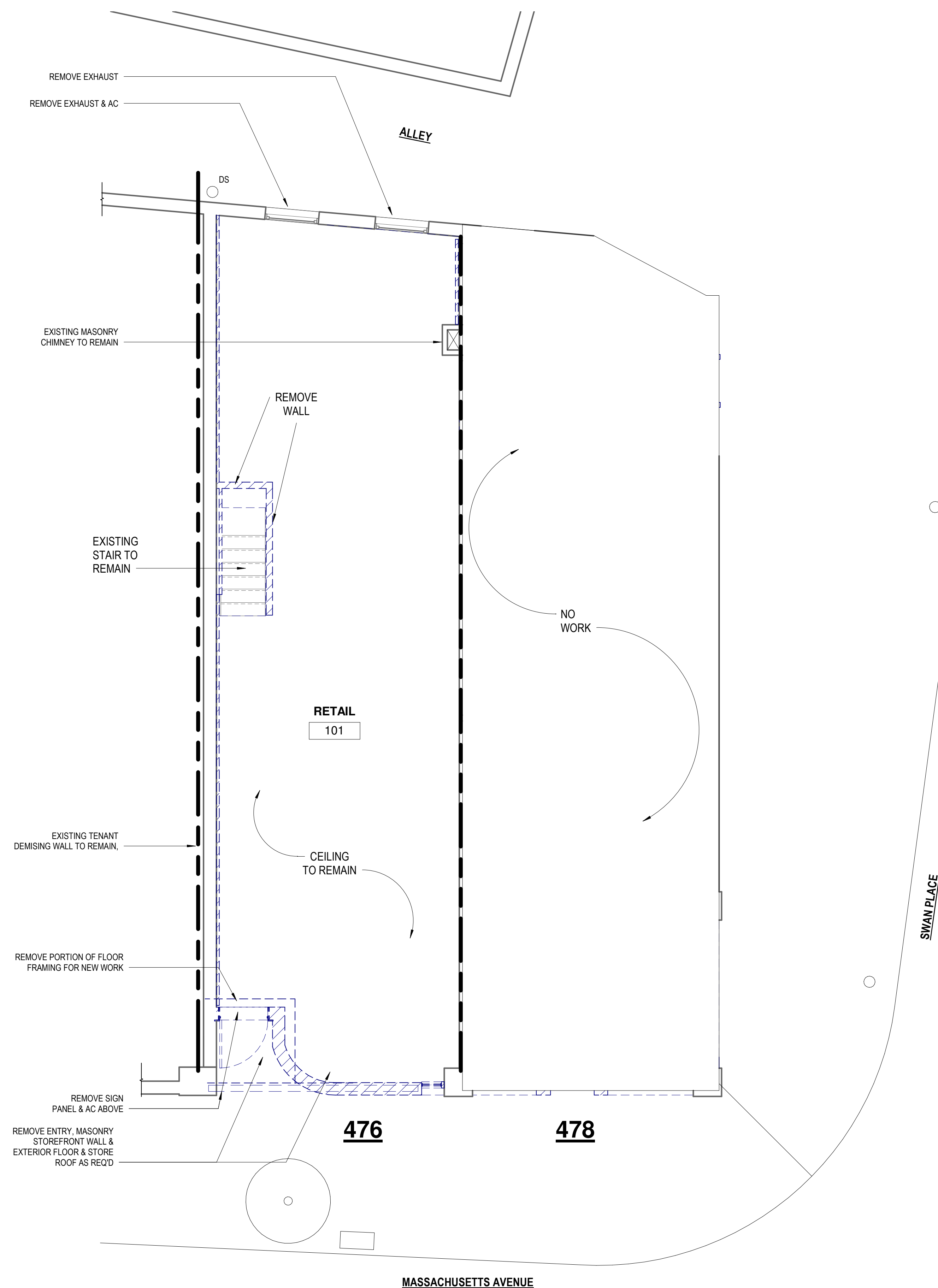
1 Demo First Floor Plan 1/4" = 1'-0"
