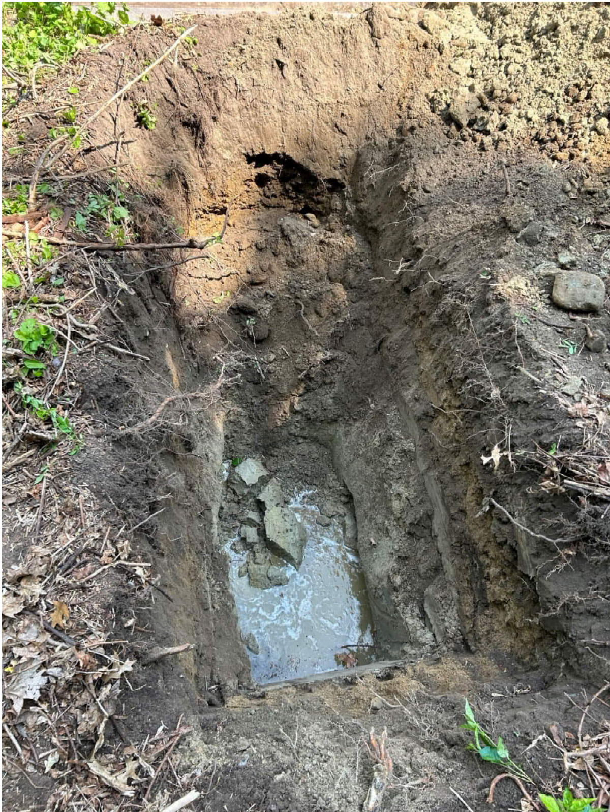
TP-5 with standing water at bottom. Note redoximorphic features on side wall.
