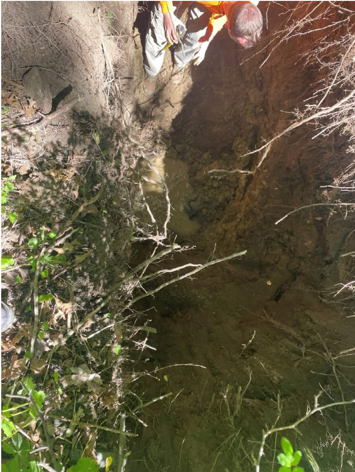
TP-3 with standing water at bottom. Note redoximorphic features on side wall.
