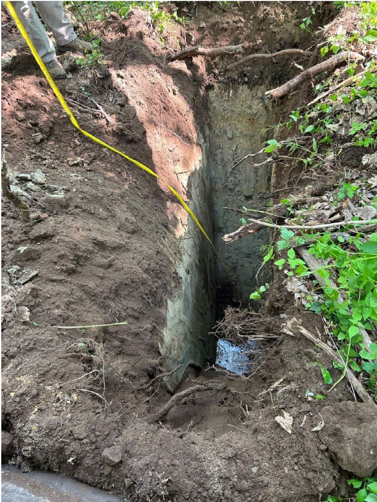
TP-6 with standing water at bottom. Note redoximorphic features on side wall.
