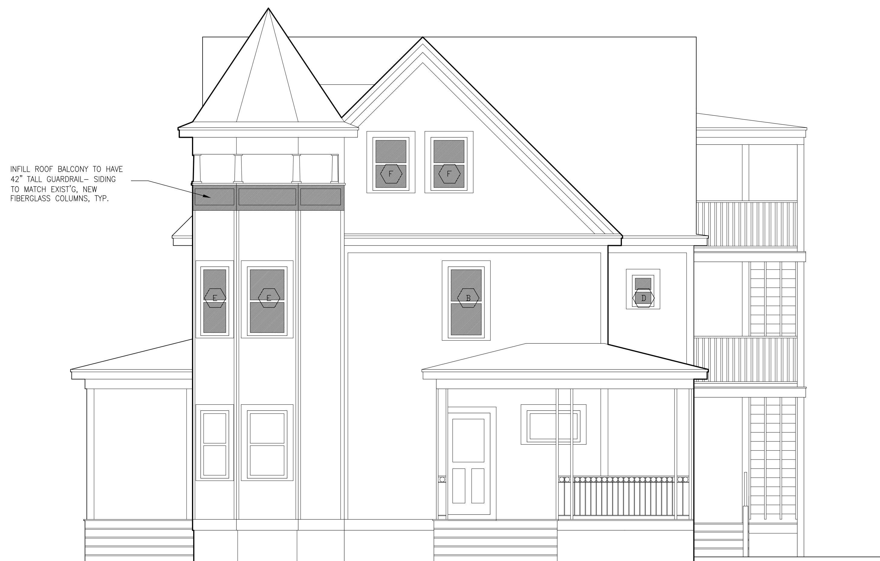
1 PROPOSED EAST ELEVATION SCALE: 1/4" = 1'-0"
