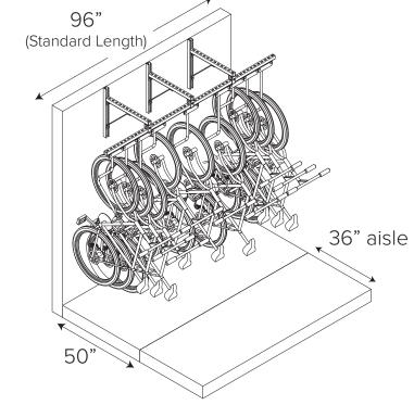
Bike Files may be lined up end to end to fill the available space. A 36" aisle should be left between the ends of bikes in racks facing one another.
