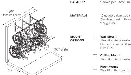
12 gauge galvanized steel trolley track Stainless steel trolley assembly 1" 16g arms
