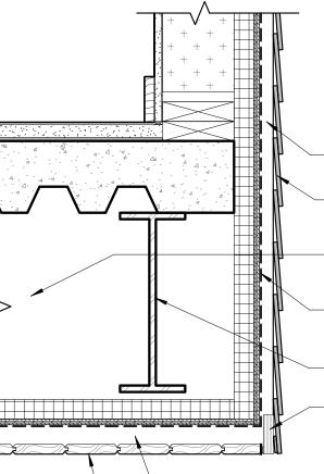
1X4 PT WD VERTICAL STRAPPING AT 16" O.C. FIBER CEMENT PLANK SIDING, 4" REVEAL
