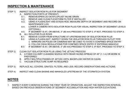
2. CONDUCT JETTING AND VACTORING ANNUALLY OR WHEN INSPECTION SHOWS THAT MAINTENANCE IS NECESSARY.
