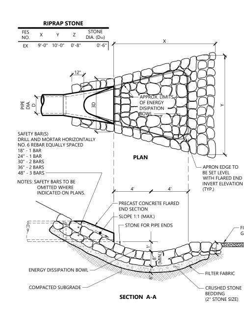
Flared End Section (FES) with Stone Protection N.T.S. Source: VHB REV
