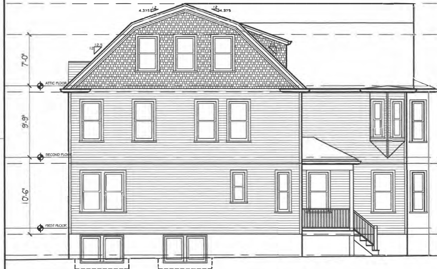
LEFT SIDE ELEVATION 1/8" = 1'-0"
