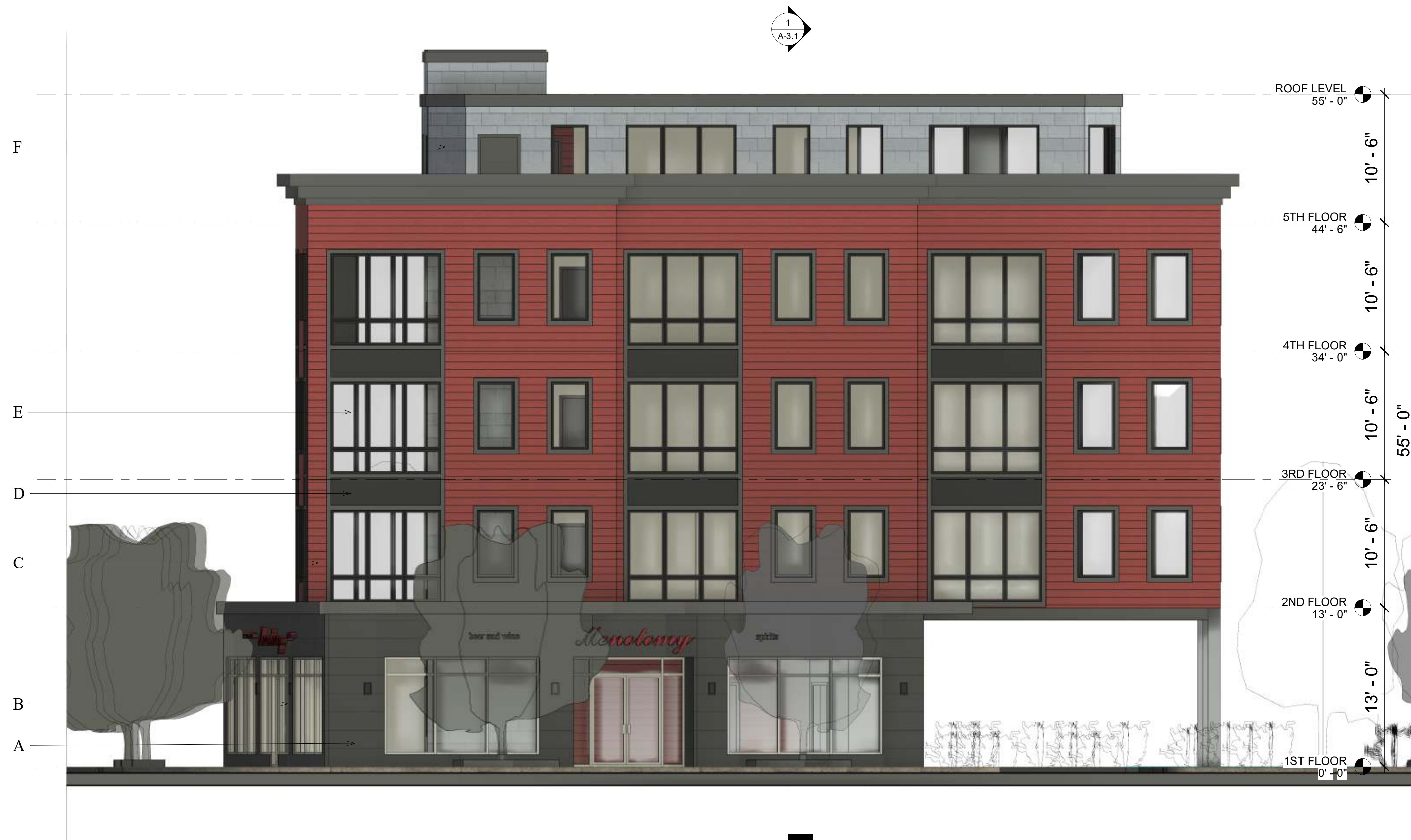
① PROPOSED BROADWAY ELEVATION 3/16" = 1'-0"
